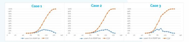
Each of these plots (blue line) give the likelihood that users are located at a place where RSRP is at a certain level. The orange line is the corresponding cumulative distribution functions for those user distributions. As one can see from real life, as most users are indoors and not outdoors we end up with very few users >-80dBm, ie the area with the 4T4R system with 1T4R had its best gains.
