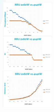
At this point, it is easy to be led astray with such a visible gain under -8odBm. The issue with graphs like this is that they give a false view of how much is covered rank 2+. The graphs easily exaggerate the area/users covered.
